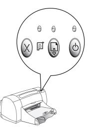
Power Button and Light – Use the Power Button to turn the printer on and off. The green light above the Power Button flashes when the printer is processing information.
